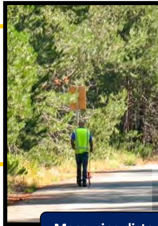
Measuring distance between manholes with walking wheel
